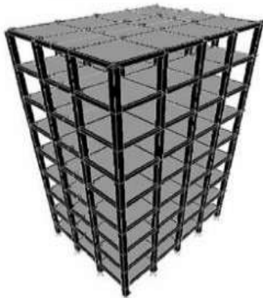
3-D view of the eight storey building (G+8) created in ETAB Gravity load
